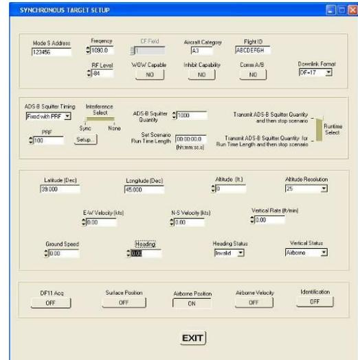
At the bottom of this screen are buttons to turn ON/OFF each type of channel 0 squitter: DF11 acquisition, Surface Position, Airborne Position, Airborne Velocity and/or Identification.
