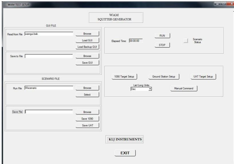
From the opening screen, select WAM (Moving Targets) to access the WAM Squitter Generator GUI shown above. From this screen, you can load and save GUI And Scenario Files, select Lat/Long Units, Manual Commands, and Scenario Run time in the same manner as with the Synchronous and Asynchronous screens.
