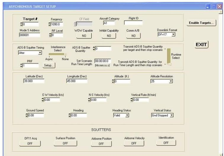
At the bottom of this screen are buttons to turn ON/OFF each type of channel 0 squitter: DF11 acquisition, Surface Position, Airborne Position, Airborne Velocity and/or Identification.
